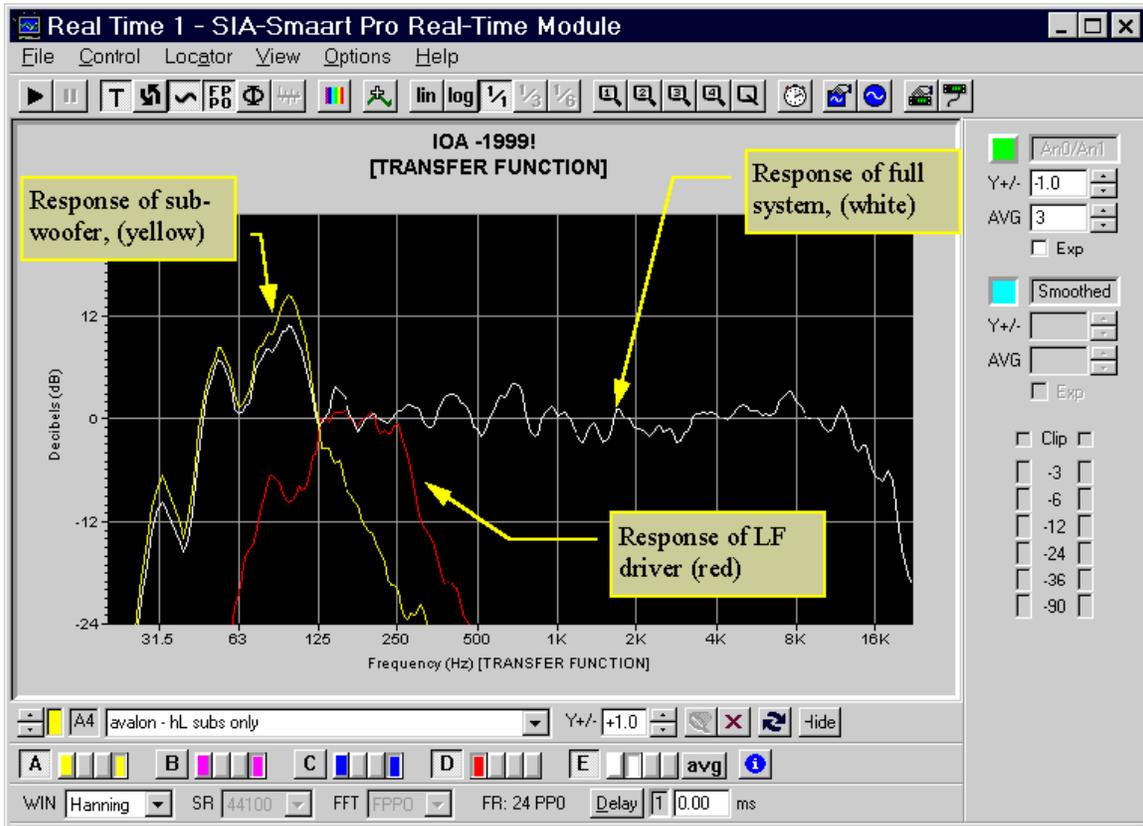
Figure #2: You can see the transfer function of the entire system, the LF drivers and the subwoofers measured separately.
