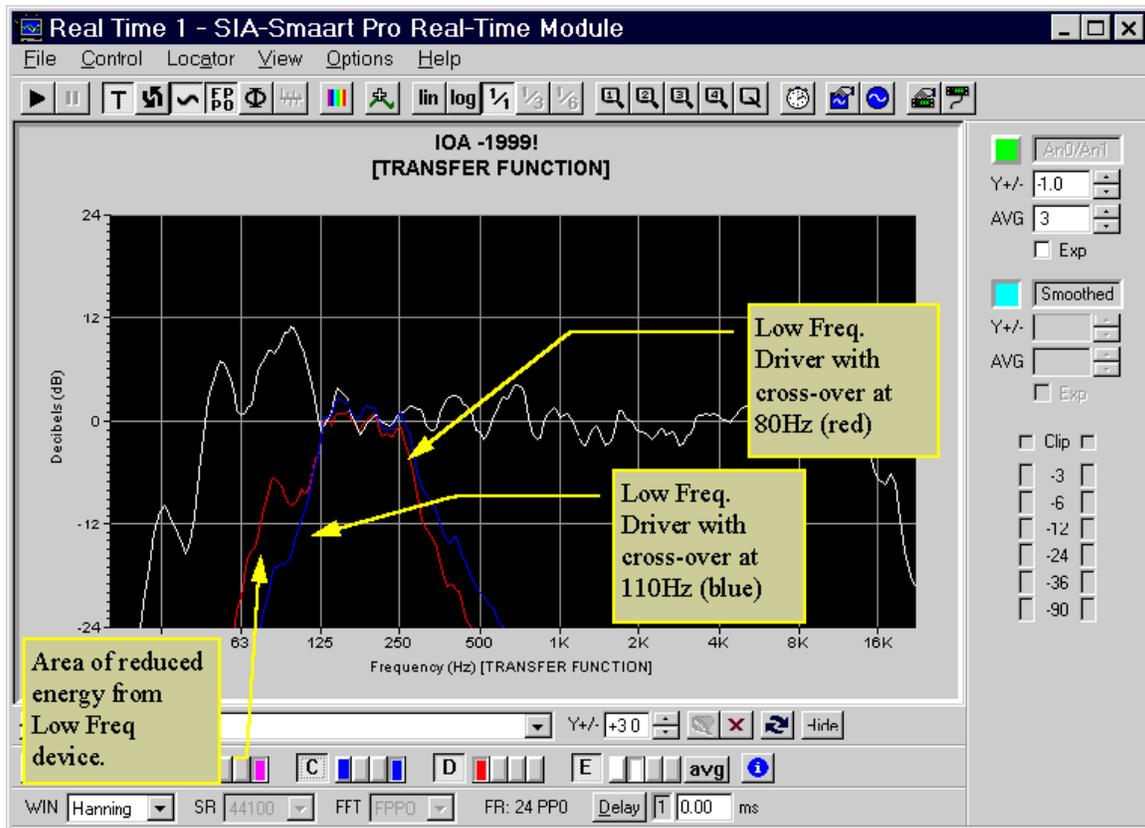
Figure #3: the full system measurement and two measurements of the LF drivers in the AVALON system. Because the subwoofers are being run at a 10 dB boost, moving the high-pass crossover point of the LF device from 80 Hz to 110 Hertz reduced the overlap between the LF and subwoofers. Less overlap is desirable when the woofers and subwoofers are in close proximity.
