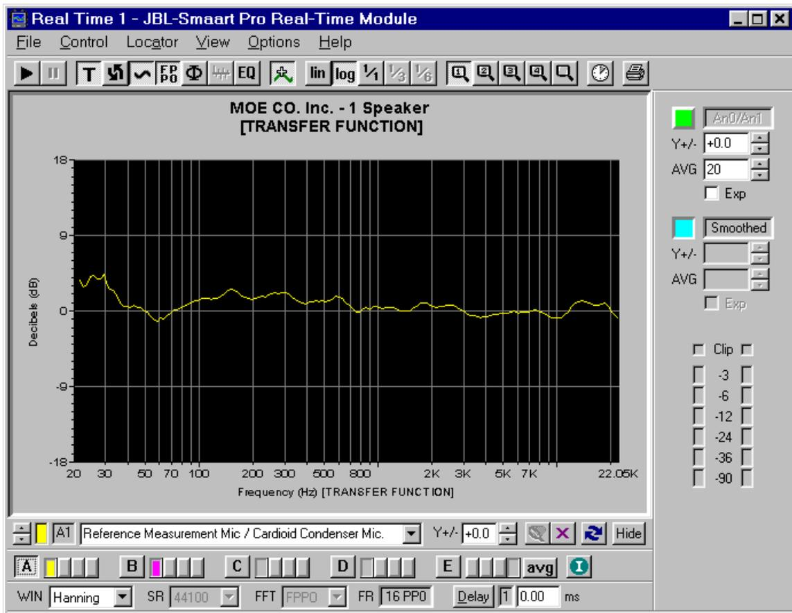
**Figure 1:** Transfer function measurement comparing a high-quality measurement microphone to a popular cardioid condenser microphone. In this measurement, the output of the measurement microphone is used as the *reference* signal and the output of the cardioid mic is the *measurement* signal.
