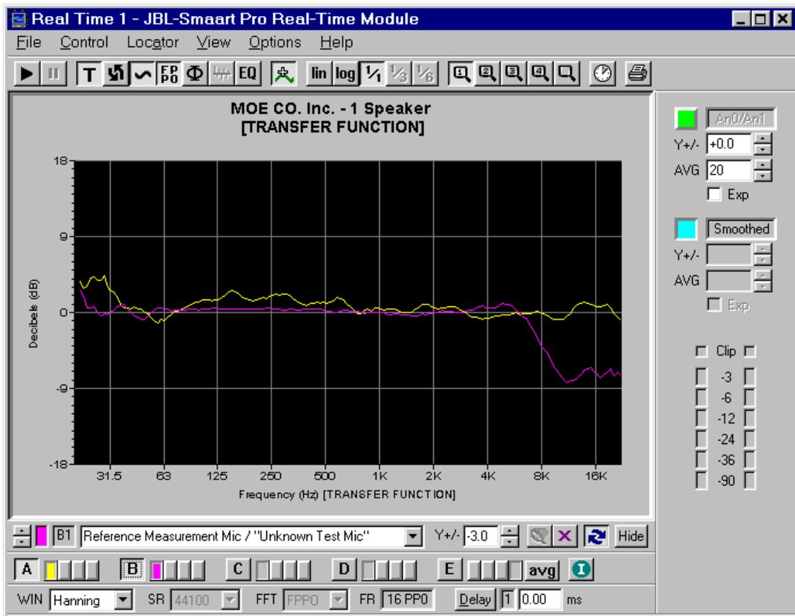
**Figure 2:** The results of the second transfer measurement (in purple) comparing the response of my reference measurement microphone to the “unknown test microphone.” Notice that in Transfer Function mode, when the 1/1 (octave) button is pressed, the grid lines and frequency labels on the graph appear at octave, rather than decade intervals.
