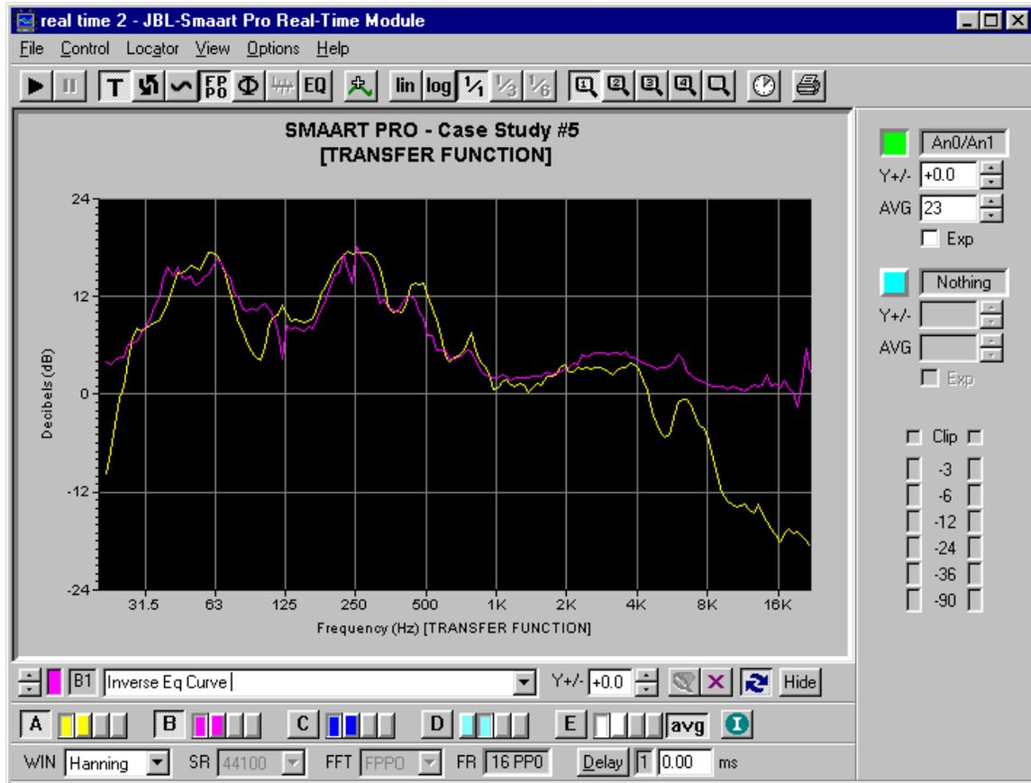
Figure 2: Inverse EQ response used to adjust system. This trace was captured sometime during the early part of the performance. Music was the noise source here which explains the relative lack of smoothness in the trace (there was not a lot of low-frequency energy present)..
