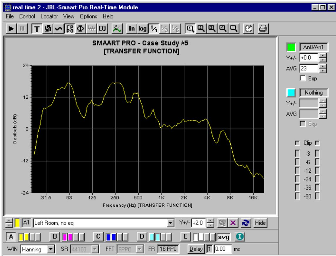
Figure 1: A Fixed Point Per Octave Resolution Transfer function measurement of the Raw system frequency response. Notice the huge low-frequency bump at 60Hz. This is a result of the stage cavities trying to “take off” (resonate acoustically). To help with this problem, I reduced the overall level of the feed to the subwoofers by 6db.
