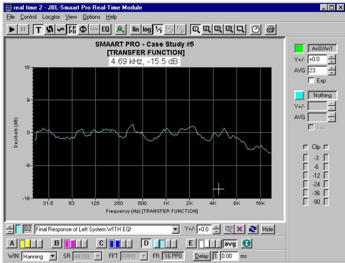
Figure 3: Frequency response after EQ — full room, microphones at the FOH mix position.
