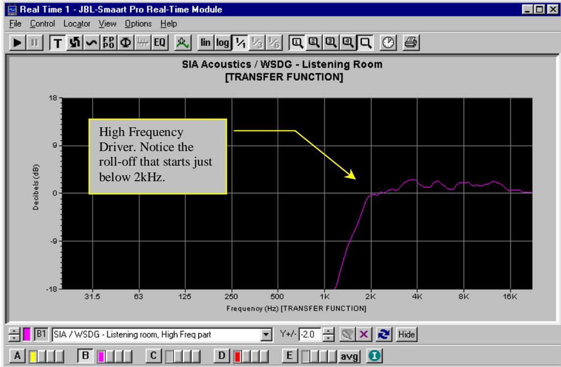
Figure #3: The high Frequency driver response. Notice the steep decay of the driver/cross-over. By looking at the two points on the decay I was able to see that a 18 dB/octave filter was used.
