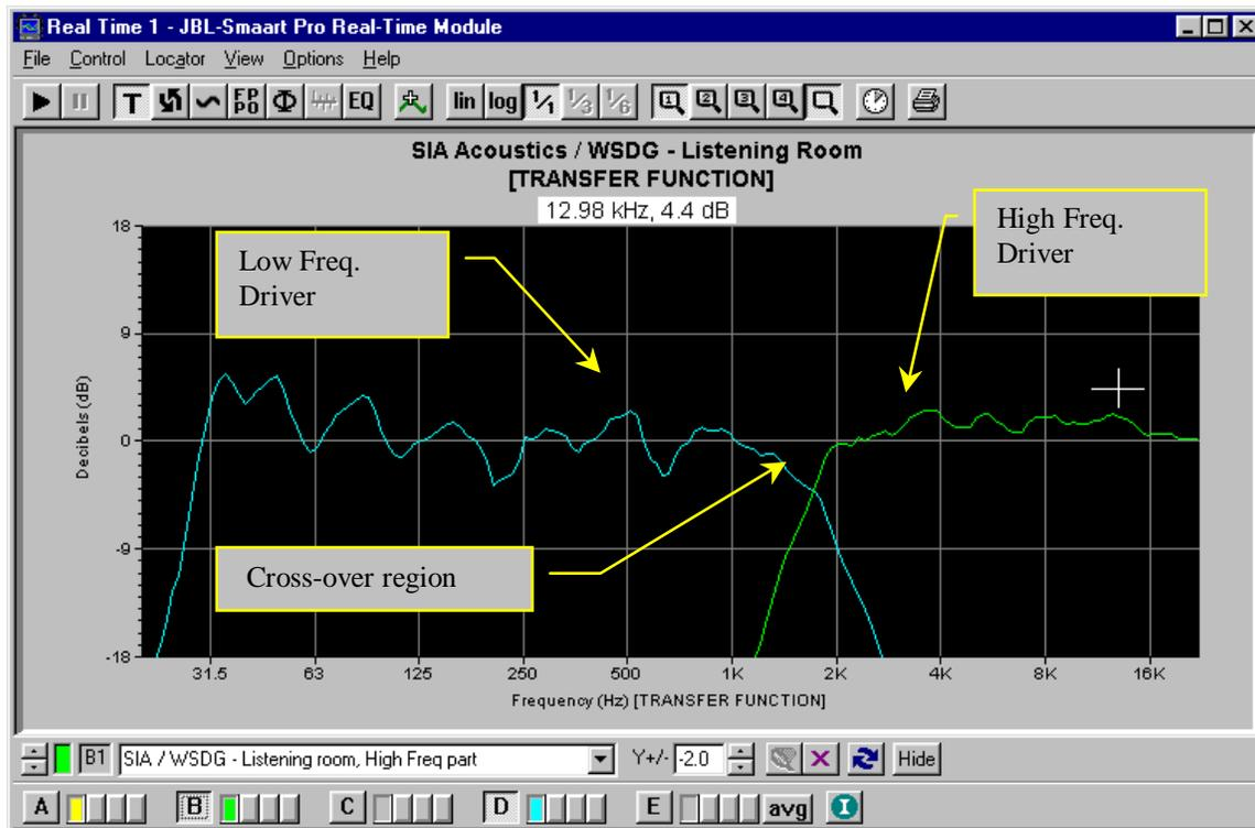
**Figure #3:** The high and low frequency drivers measured independently. By measuring each driver independently and overlaying their response curves, it is easy to see how the crossover filters are set to provide optimum overlap and response. This approach is particularly useful for setting crossovers and relative amplifier levels.
