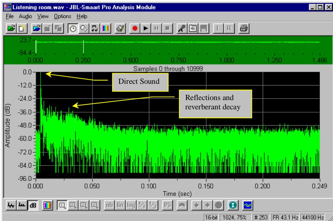
**Figure #1:** The impulse response of a single 2-way loudspeaker measured about 4' from the loudspeaker, using a 44100 Hz sampling rate, 65536 point FFT, and 4 averages (frames).
