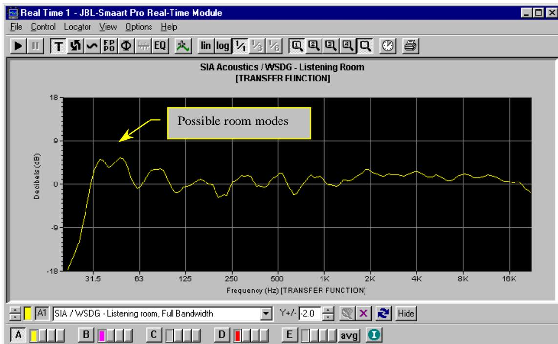
**Figure #2:** The transfer function of a single two-way loudspeaker measured in a listening room. Notice that the speaker seems extremely well behaved above 125 Hz. Below 125 Hz., interaction with the room dominates the measurement.
