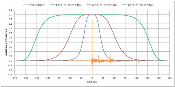
The chart below shows equivalent FTW time window functions for 10%, 25% and 50% half window sizes relative to a 16K FFT.
