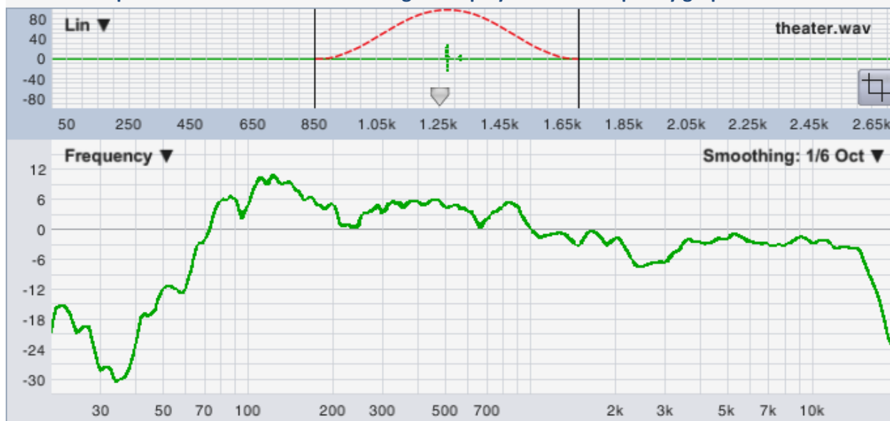
Figure 134: Moving the time 0 point and selecting a time range for display. The time range selected in the navigation pane applies to the Frequency graph as well as time domain graphs (Lin, Log or ETC). Note that Smaart uses a tapered data window when transforming any subset of the full IR time range. We've drawn the outline of a Hann window in red on the navigation pane of the "result" portion of the illustration above to help visualize this.
