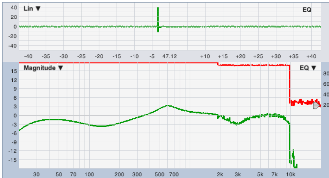
Figure 112: HF coherence loss in the MTW transfer function due to delay mismatch
