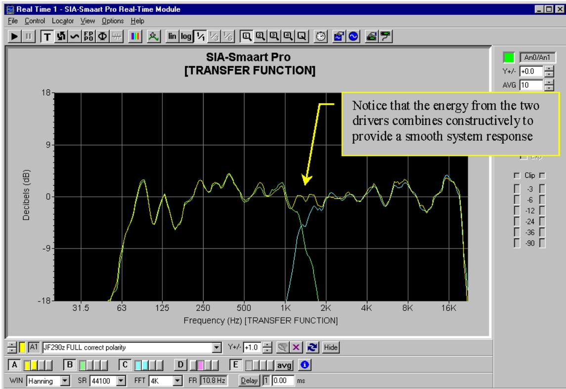
**Figure #4:** Frequency response of High Frequency (HF) and Low Frequency (LF) drivers in a JF290z measured separately (green and cyan traces) and together (yellow trace). Notice how the energy from the two drivers interacts constructively to provide a smooth system response (i.e. the response of both systems adds to ‘fill the hole’ at crossover).
