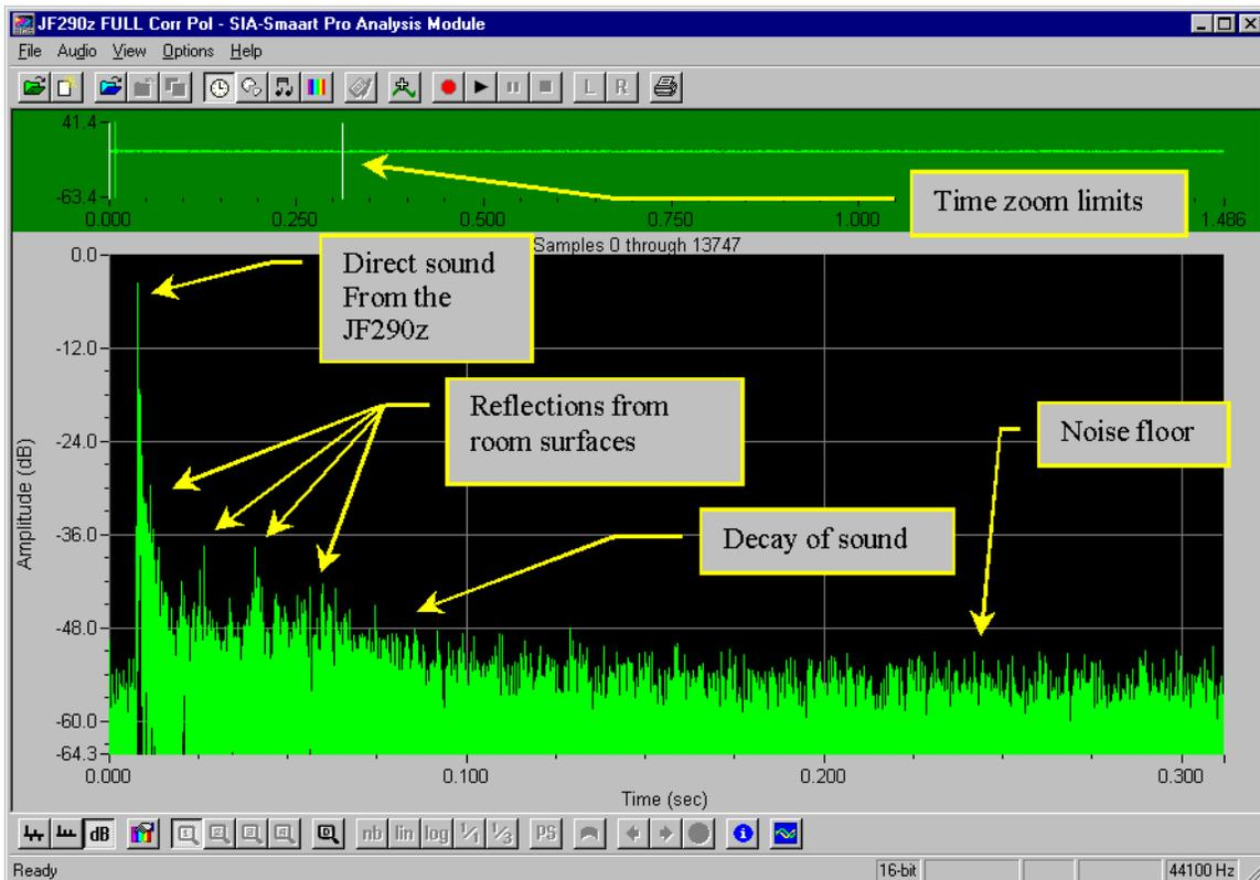
**Figure #1:** The impulse response measured by the Smart's delay locator, displayed in Smart's analysis module. Note the strong direct sound and the lower level of the visible reflections. A 64k FFT and 44.1kHz sampling rate with 3 averages were used in the delay locator.
