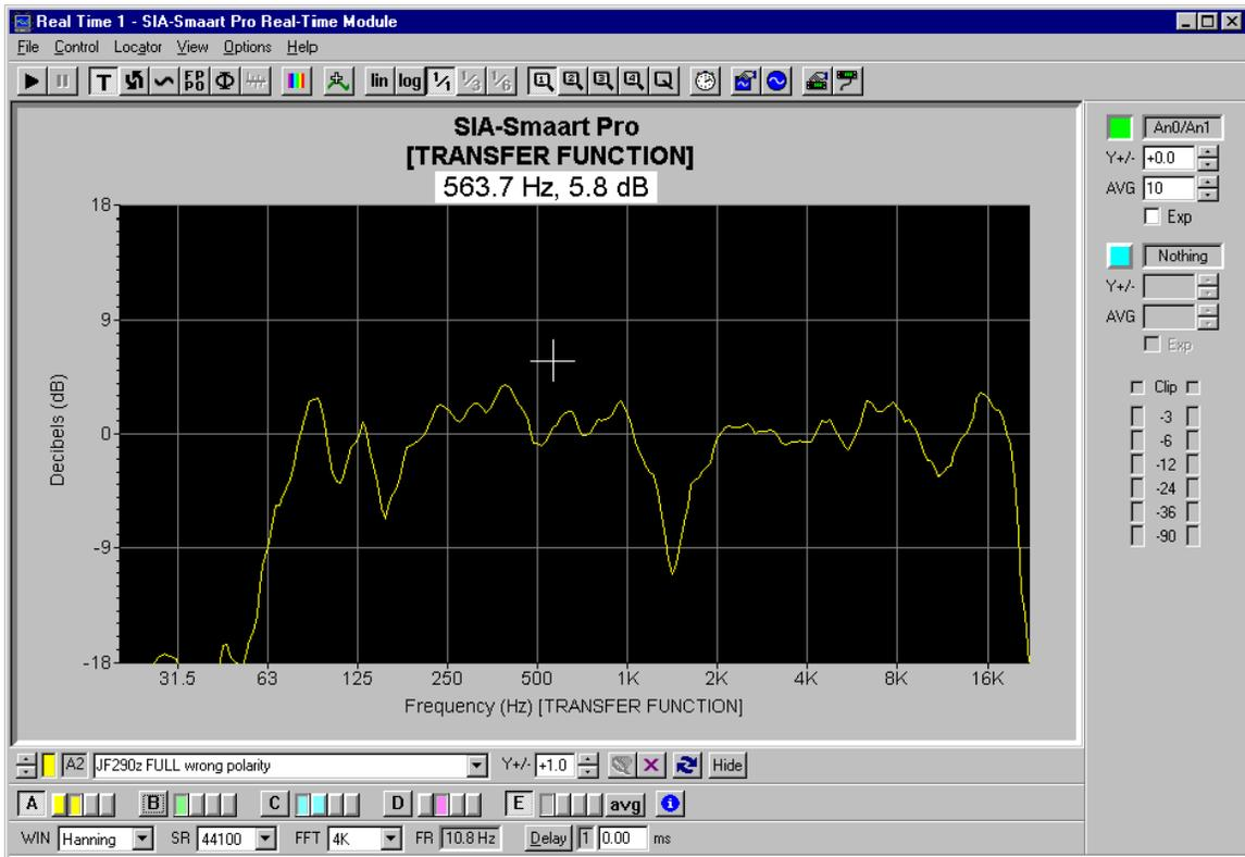
**Figure #7:** The frequency response of the loudspeaker with the polarity of the HF driver flipped (relative to the LF driver). Notice that the energy from the two drivers no longer adds constructively, creating a hole at the crossover frequency. This hole is clearly audible in vocals and other upper-mid range energy when listening to the speaker mis-wired.
