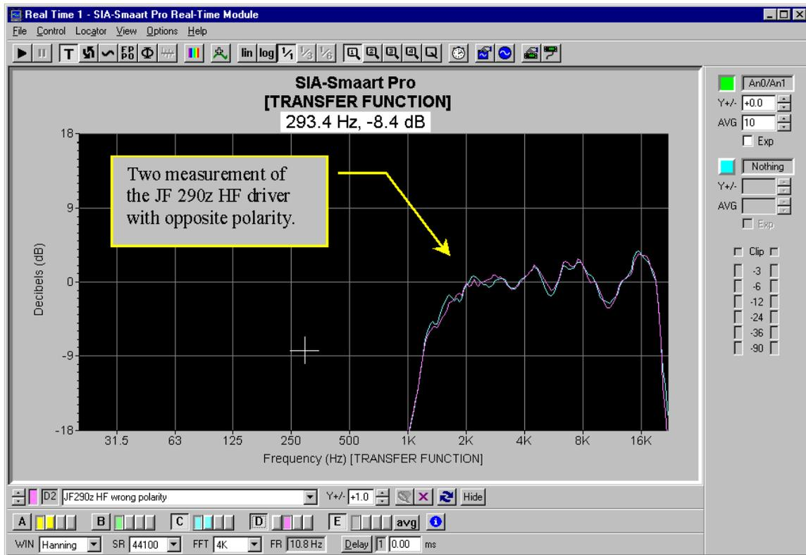
**Figure #6:** Two measurements of the HF driver alone. Notice that even though the polarity is positive in one measurement and negative in the other, the frequency response is almost identical. Any small differences can be reduced (or even eliminated) by increasing the number of averages for each measurement.
