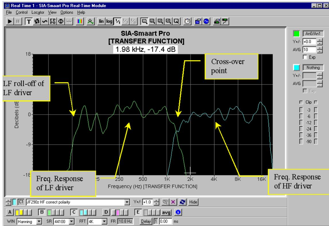
**Figure #3:** Frequency response of High Frequency (HF) and Low Frequency (LF) drivers in a JF290z. Note the roll-offs of the LF and HF drivers meet at  $\sim 3$ B. Again the gently smoothed FPPO transfer function was used.
