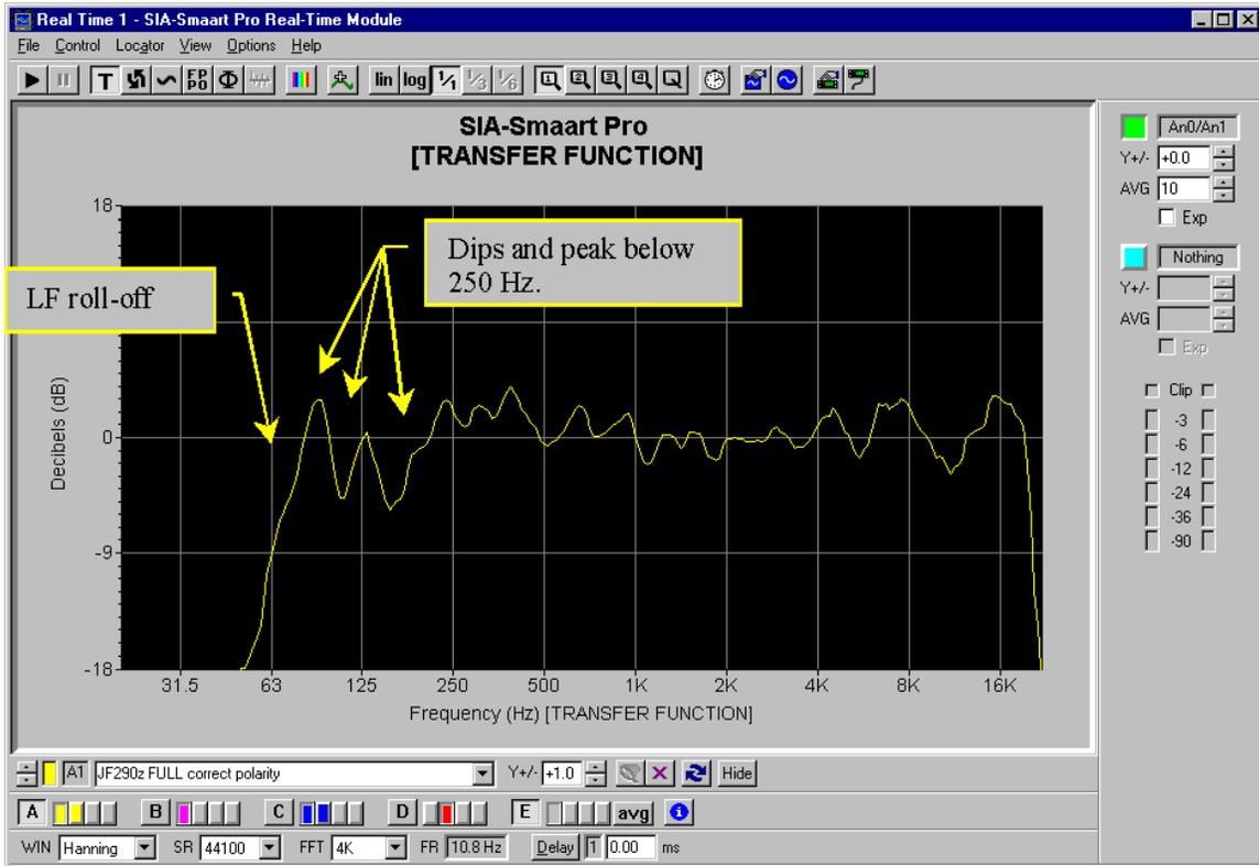
**Figure #2:** Frequency response of the EAW JF290z measured using a gently smoothed FPPO (fixed Point Per Octave) transfer function. Pink noise was used as a reference signal and 10 averages were included in the measurement. Notice that the speaker is extremely flat in the 250 to 16kHz frequency range. Below 250 Hz there seem to be two dips and one peak. The Low frequency roll-off of the loudspeaker is visible.
