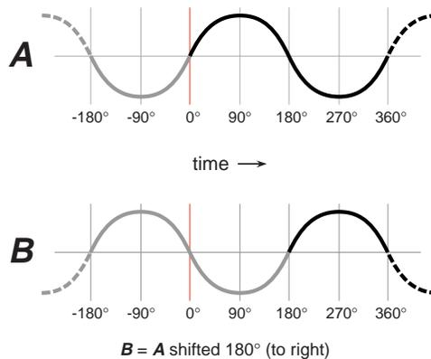
**Figure 5:** The figure above shows two sine waves. In part A of the figure a standard sine wave is shown. Notice that relative time is shown in degrees with each 90 degrees of shift equaling a quarter wavelength. In part B of the figure the sine wave has been shifted to the right by 180 degrees. Notice that the wave in part B is the same as the wave in part A only with opposite polarity (positive vs. negative).
